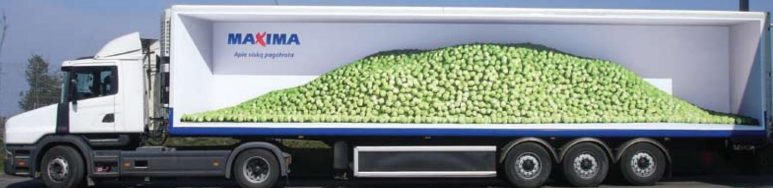
Soft-sided graphics is a viable niche, especially for clients that need to swap out their graphics frequently. Rather than PSA vinyl, soft-side applications use a banner material that is held on the truck using a framing system. (Image courtesy of TruckAds)
