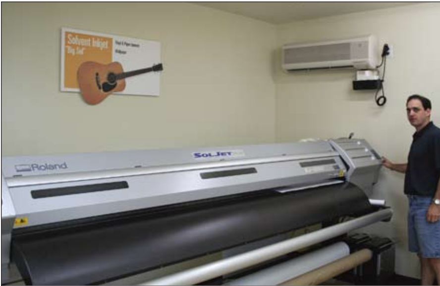
Here is our 102"-wide Roland SolJet Pro II SJ 1000 solvent-based printer. We have another one of these babies that has been set up to run with dye sublimation inks.
