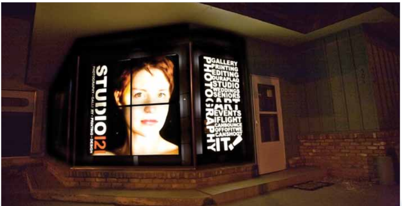
Mark Lewis, who owns Studio 121 in Loveland, Colo., created this storefront backlit display for his studio with six light boxes stacked together (four in one window and two in the other). He printed the images on LexJet TOUGHcoat Water-Resistant Polypropylene on his aqueous Epson 9880 printer. (Image courtesy LexJet)
