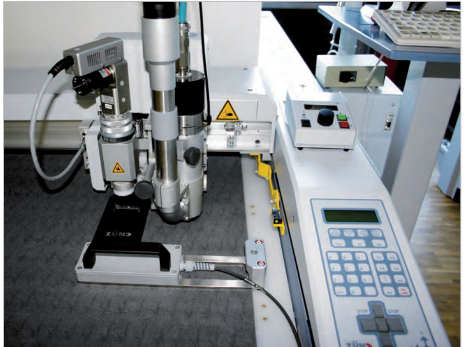
The AKI-2 Tool Manager system available on Zünd cutters allows for easy switching of cutter tools. (Photo courtesy Zünd)
