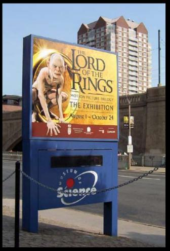
A backlit such as this one that must look crisp when lit at night and unlit in daylight can be created on a white-ink capable flatbed printer by printing colors followed by a layer of white followed by colors. In daylight the eye sees only the white and outer layer of color. At night the inner color layer brings the added density needed for a good backlit image.
