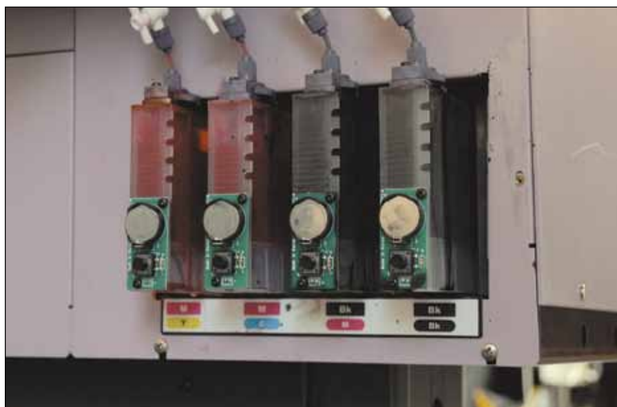
Here is a close-up of the reset buttons. One is required for each ink channel.
