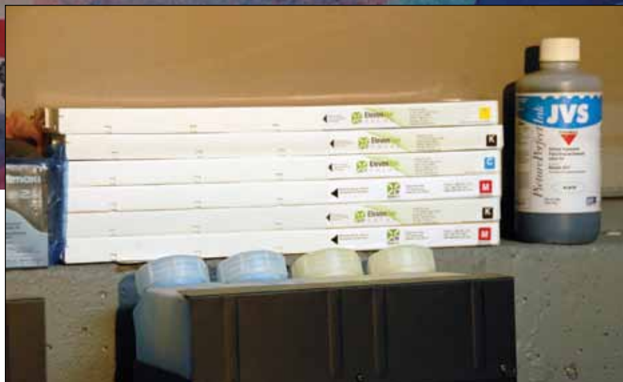
Ink replacement systems are available in cartridge form, or in bulk ink feed systems.
