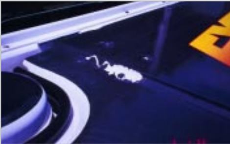
In these examples the installer failed to cut the vinyl around bolts and rivets. When a pressure washer was used to clean the vehicle on the left, it blew out the vinyl. The other job simply looks very poorly done.
