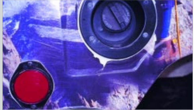
If graphics are wrapped around the gas cap, the area must be thoroughly cleaned and edge-sealed to prevent fuel from lifting the film as in this example.
