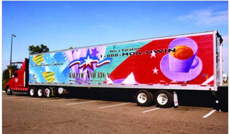
Vehicle graphics made on e-stat machines (such as this one), require a transfer process and have traditionally been protected using film laminates. Some shops are using liquid coatings on e-stat vehicle graphics. (Photo courtesy of 3M)
