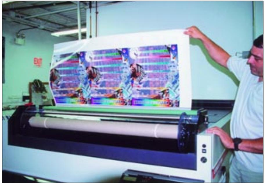
Prints off of the photo writer cost about 30 cents per square foot to produce. The machines can easily produce more than 200 square feet of output per hour at 4,000 optical dpi.
