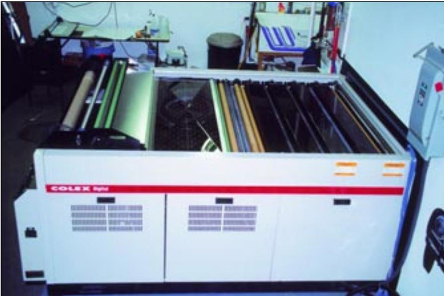
The photo processor can crank out 60 inches per minute of finished prints that require no lamination.
