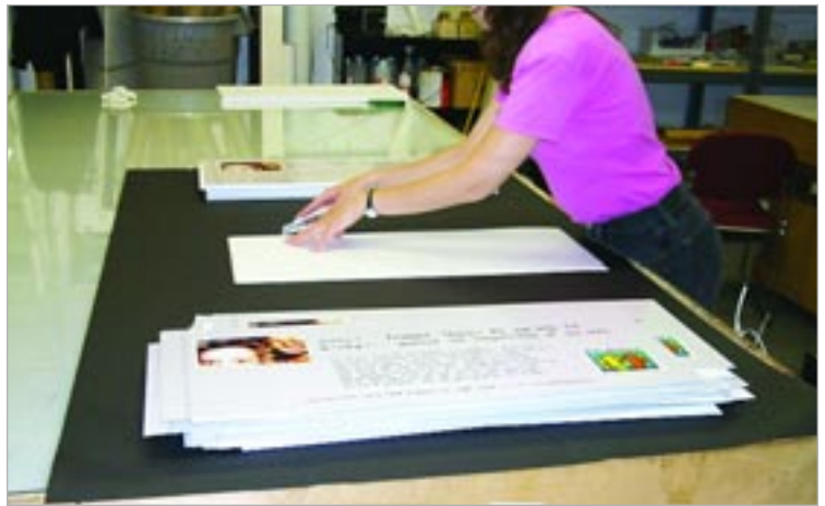
After the Lambda print has been mounted, overbleed (excess paper print with adhesive) is trimmed away.
