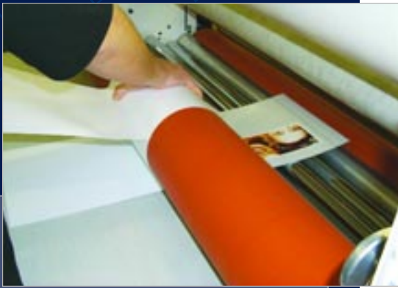
A Lambda print is mounted to .040 polystyrene for a bus interior — a typical interior bus graphic application.
