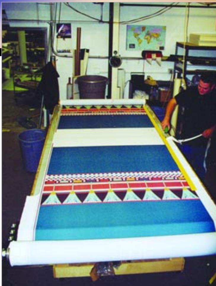
Once printed and sublimated, dye-sub graphics result in very nice color intensities. In sublimation the dye vaporizes and bonds directly to the polyester fibers.
