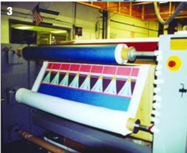
One of the trickier aspects of working with dye sub is the fact that colors entering the heat press (images 1 and 2) look drastically different than the colors coming out (image 3). Carefully cataloging color profiles for your output, as was done with this design printed onto hercules material, will help you match clients' color needs.
