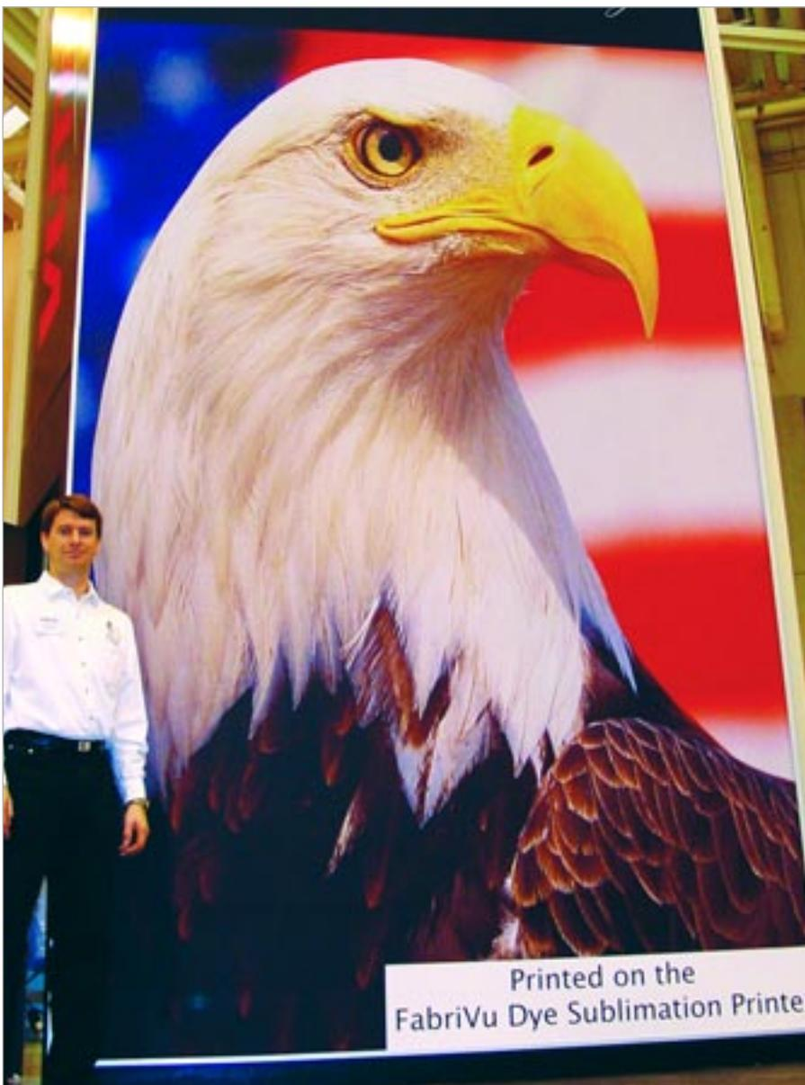
This print was done using the traditional method of printing onto a transfer paper and then sublimating it onto fabric. Sublimation allows inks to bond permanently with the polyester fibers.
