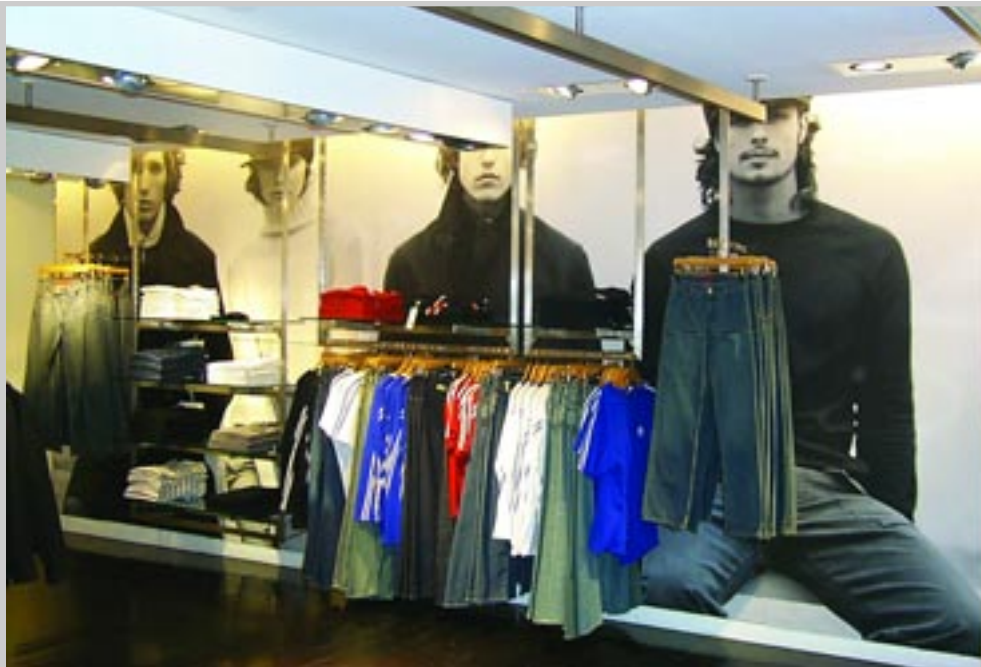
Here is an interior wall wrap. Although UV was of little concern, the main durability issue was from people touching and picking, clothing racks being banged against it, and general retail abuse. (Photo courtesy One Source, New York City)
