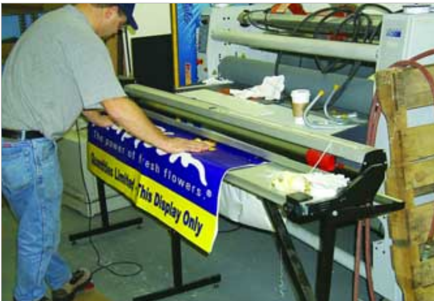
Rotary cutters, such as this one from Rotatrim, are ideal for cutting paper, banner and adhesive-backed vinyl.
