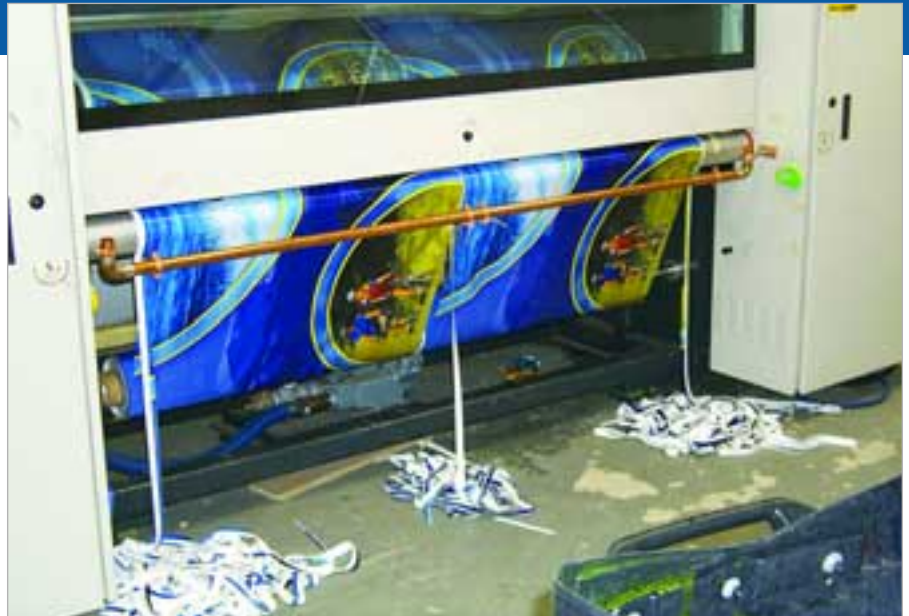
This is a six-bladed in-line slitter that we created to fit onto the back of our NUR Fresco printer. Parts were obtained at Home Depot for about $52, and it saves us about $900 a week in labor costs.
