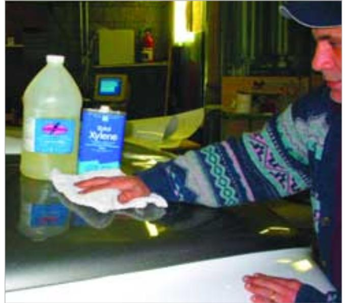
To remove adhesive residue we use a number of chemicals, including a citrus-based stripper called Rapid Remover that will not hurt the paint or plastic parts of the vehicle. A much stronger agent, called Xylol Xylene, can be used, but it is more dangerous because it is flammable and the vapors can be harmful.
