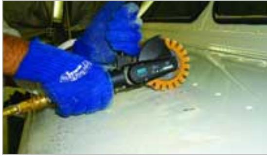
We've had great success using the MBX Vinyl Zapper. It's ideal for removing cut vinyl letters. It works quickly and doesn't leave an adhesive residue behind.
