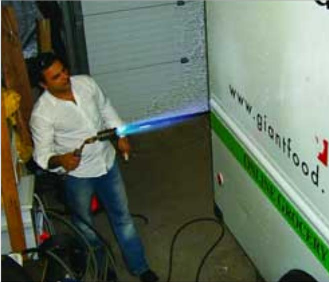
When it comes to removing vinyl, heat is your friend. Heat from an acetylene torch can be used to soften the adhesive making removal easier. However, *extreme caution* is advised. The key is to heat the vehicle without burning the film — or the vehicle.
