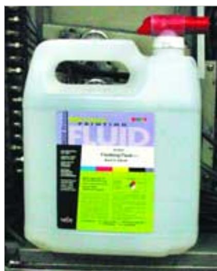
Solvent ink printers use a flush procedure that allows the operator to switch from ink to a solvent solution that can be run through the printheads for internal cleaning. Special flushing fluid is available for specific printers from some manufacturers.
