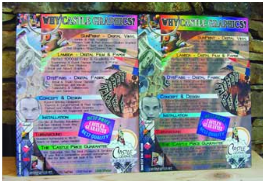
The image on the left was printed directly onto high-quality DiBond with a UV-curable flatbed printer while the image on the right was printed with a Lambda and mounted to Gator board. The photo was taken from approximately two feet away.
