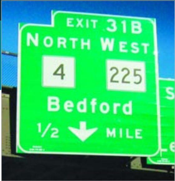
Reflective vinyl with permanent adhesives are often used on municipal signs. These babies last a long time.
