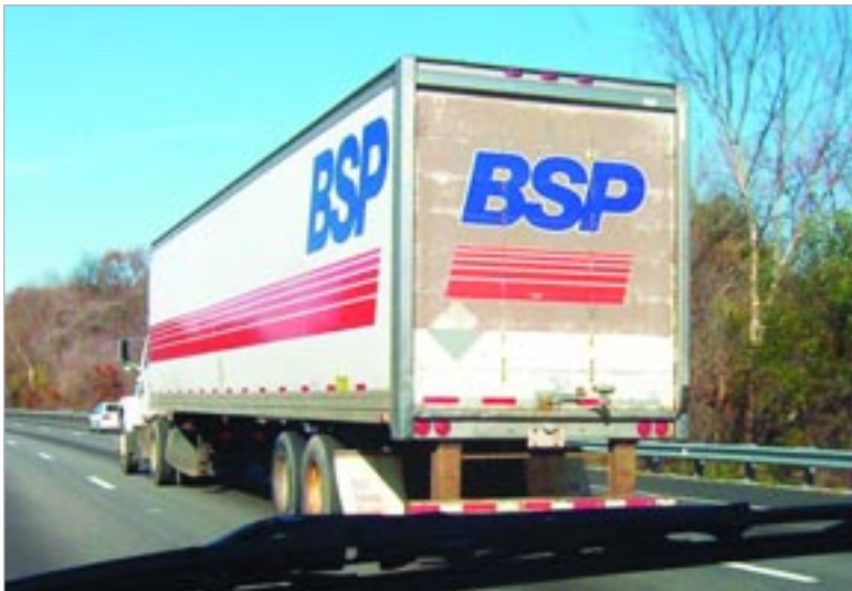
Just look at this. The paint on the back of this truck failed before the cut calendered vinyl that covers it. Vinyl is final, baby.
