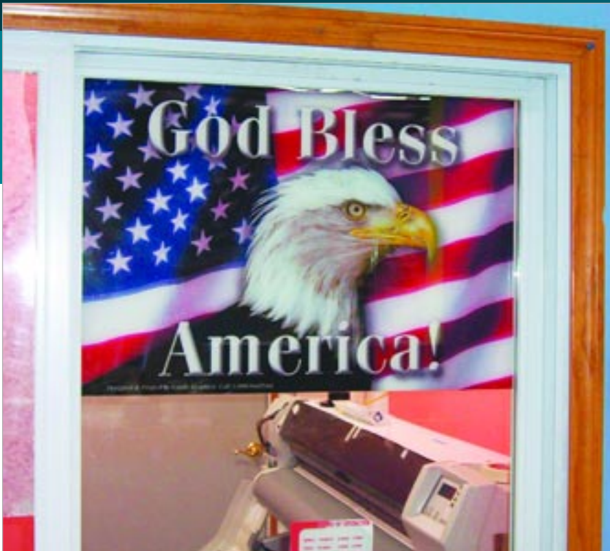
This is a reverse-printed window graphic. It's mounted on the second surface using Catalina Plastics clear calendered film, backed with Avery's 4000 series cast cut vinyl. By day it's a graphic image and by night it's a backlit display when used with a halogen light source.
