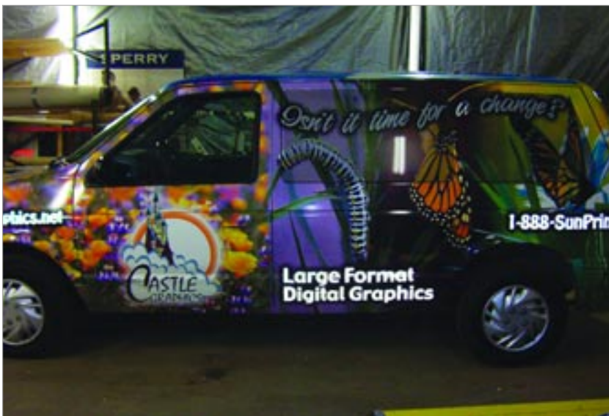
This shop truck is covered with Avery MPI 1005 EZ cast vinyl with ClearFocus window perf and Avery A7 Reflective High performance vinyl used in the white areas.
