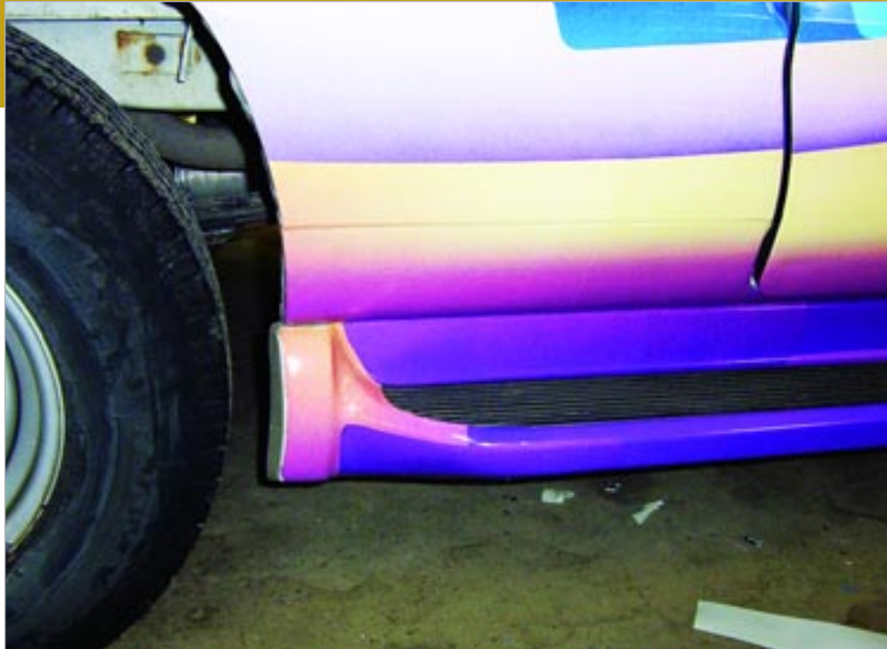
Really tight curves, like those on the running board of this vehicle, require a very stretchable film, such as Avery EZ film.
