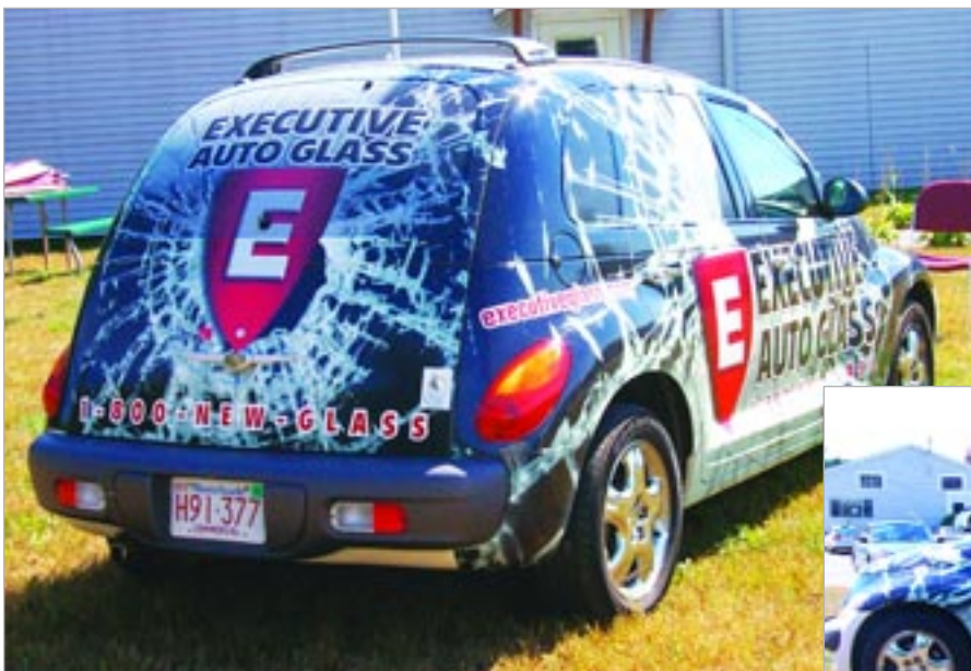
Typically, passenger vehicles, such as this PT Cruiser, are difficult to wrap because of the multiple compound curves.
