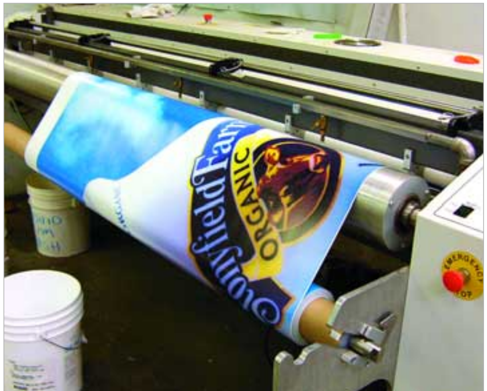
Seal's AquaSEAL SW-3000 laminator may be pricey for some shops, but it's a workhorse. The machine uses an infra-red and blown-air drying system.
