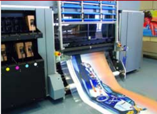
White is ideal for all types of applications on clear substrates, such as the clear film being printed to here with the white-capable Durst Rho 160W.
