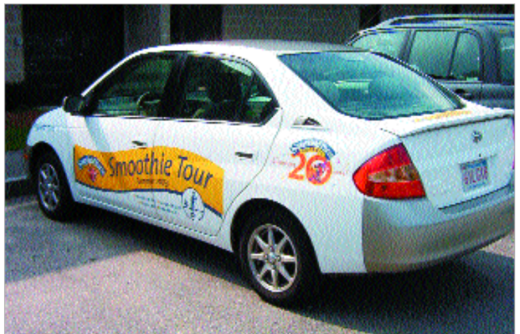
Although I generally do all my vehicle wraps using high-quality cast film, for short term applications (around 30 days), calendared film works great.
