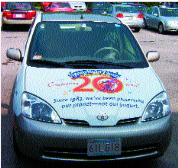
Although I generally do all my vehicle wraps using high-quality cast film, for short term applications (around 30 days), calendared film works great.
