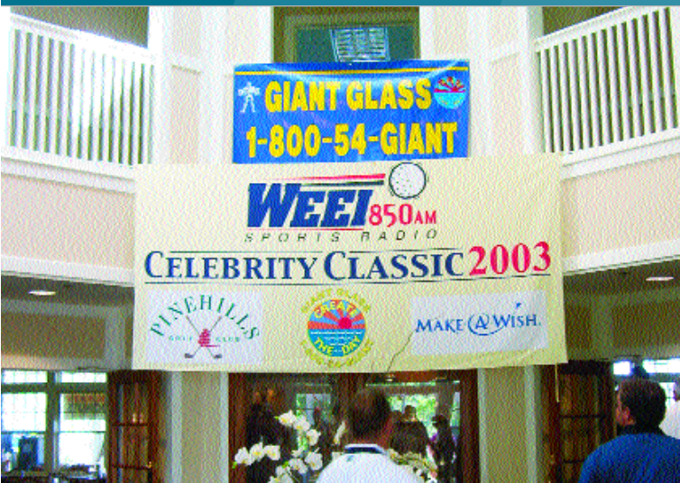
Here are two banners used together. The top banner is made from a blue banner blank with yellow cut vinyl. The lower graphic is a dye sublimated fabric banner printed onto denim light fabric.
