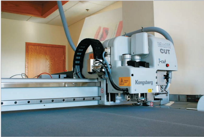
The Kongsberg MultiCut toolhead features a routing tool and a cutting tool, and also does automatic leveling.
