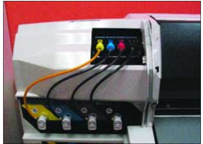
Many common aqueous-based inkjet printers are equipped with disposable thermal inkjet printheads, and manufacturers, such as Hewlett-Packard, often provide a printhead cleaning cartridge along with their bulk ink system. When the bulk ink cartridge is empty, you dispose of everything — the head, the cleaning cartridge and bulk containers and start fresh.
