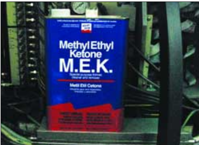
Methyl Ethyl Keytone (MEK) is a great universal solvent that can be used to efficiently clean ink from internal areas of the printer. Be careful to work with good ventilation, however, because this stuff puts off some harmful vapors. Note: do not use MEK on rubber or plastic components as the solvent tends to dissolve things.
