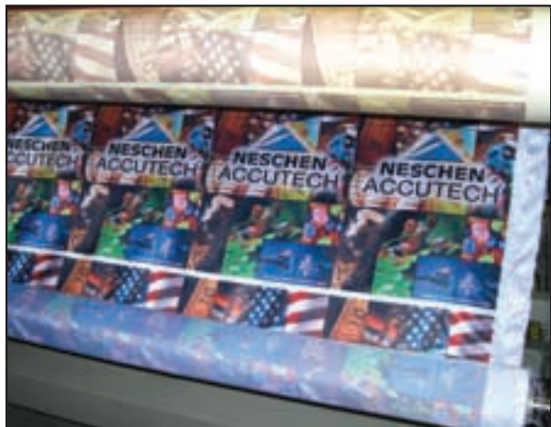
Above, carrier paper printed with a dye-sub image in reverse and uncoated fabric are fed together into the dye sublimator. The carrier paper holds dyes in place while they are sublimated into the fabric at 400 degrees F (below).
