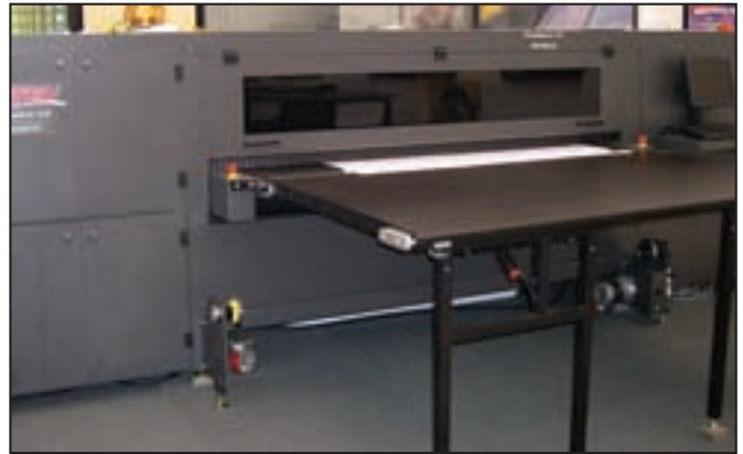
The Vutek Press Vu UV 200-600 prints UV-curable inks directly to coated or uncoated fabrics.
