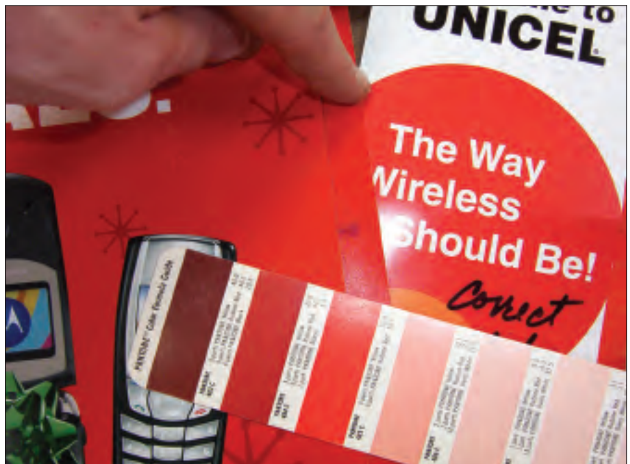
Pantone book page showing the correct color for Pantone, this page with the correct color chip being laid on the job to compare color.
