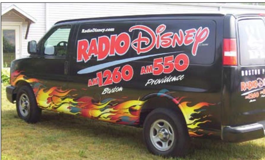
There are a number of areas on the vehicle that you must keep text away from, like door handles, front windows, name plates, license plate areas, key holes, bumpers, deep compound curves and items that could block the message.
