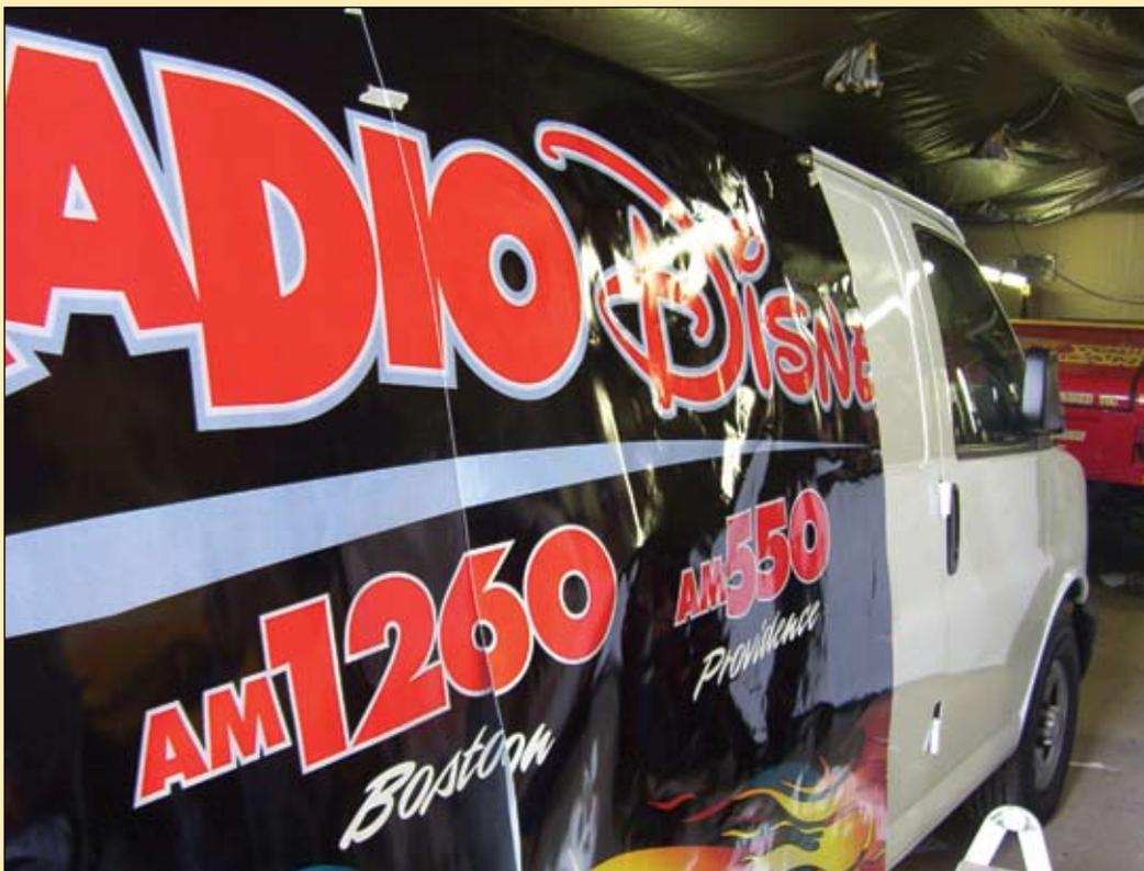
With a 2" bleed on all sides, begin laying out the panels on the vehicle to make sure the film was printed at the correct size. Tape the panels onto the vehicle with masking tape. When you are satisfied that the panels will fit correctly, begin applying, starting from the back and working toward the front.
