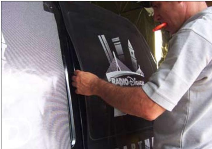
The final part of the wrap is the window perf. You must cut out all the vinyl on the glass and remove it. Line up the window perf with the graphics, and apply.
